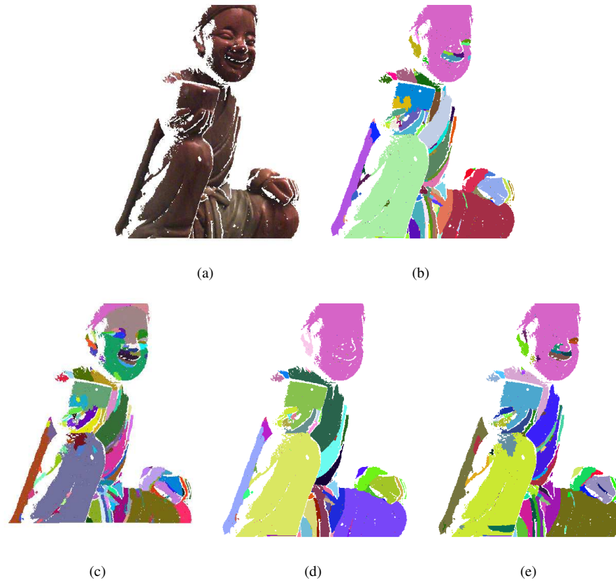
Fig. 4. Influence of the input parameters. Original range image(a). Segmented images: (b) using the same input parameters of the repeatability and correspondence test, cutting criterion threshold (c) reduced in 20% and (d) increase in 20%, and (e) 40% reduction in neighborhood radius R .
